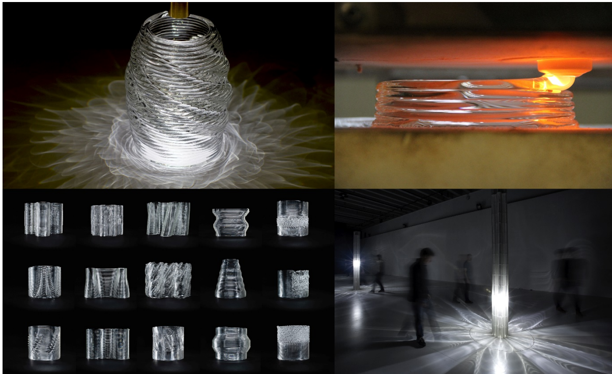
Figure 2: Additive manufacturing of optically transparent glass by the Mediated Matter Group, MIT Media Lab. Glass object with caustic pattern (top left), 3D printing process (top right), variety of printable objects (bottom left) and glass column with inserted light (bottom right) (all images courtesy of the Mediated Matter Group).
