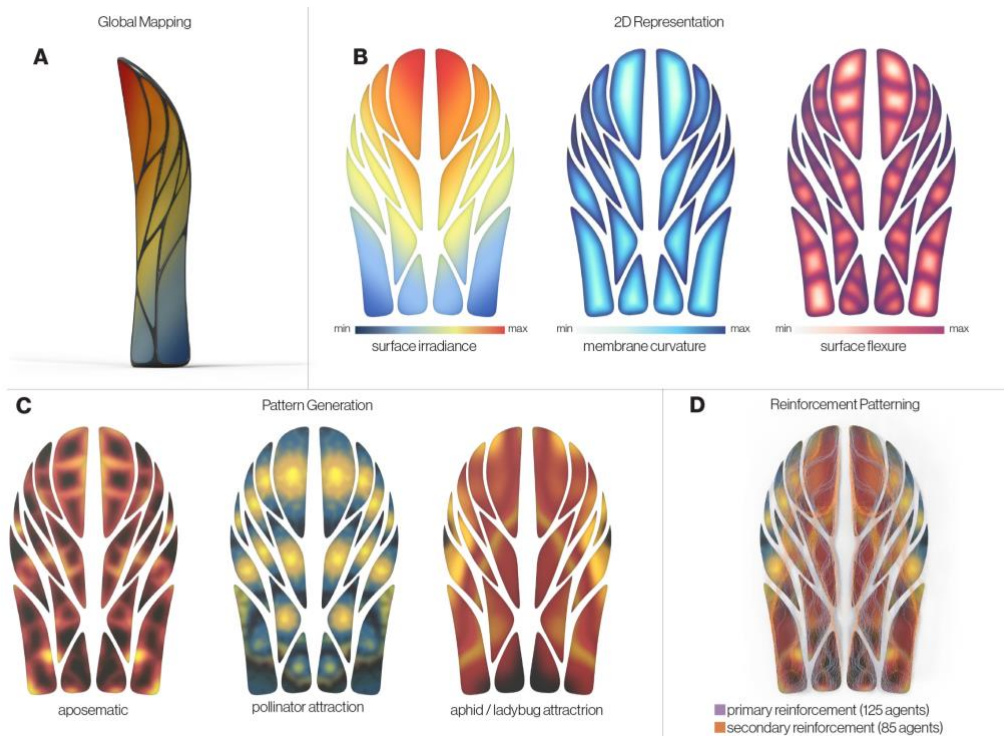
Figure 4: Environmental data associated with global scale is modeled for structural irradiance, panel membrane curvature, and surface flexure for the structure in its assembled state (a). Global maps are translated into 2D representations (b) that guide the distribution of material and color for flexible membrane elements (c) and semi-rigid reinforcement patterns (d).
